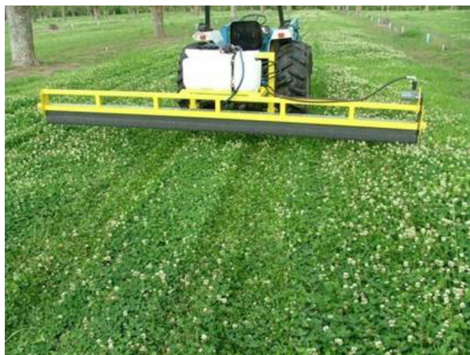
Figure 8. Weed wiper used for broadleaf weed control in orchards utilizing clover as an orchard floor cover (Photo: Bill Goff, Auburn University).
